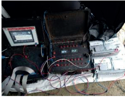
Figure 55: Baseline is tested for tightness in Høje Taastrup (Source: Gquadrat)
