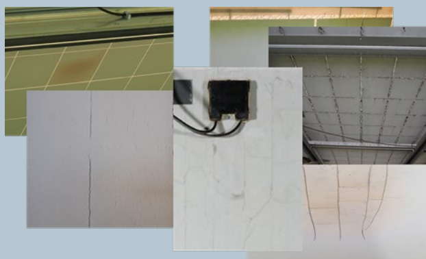
PV modules with defective back skins, photo: OFI
