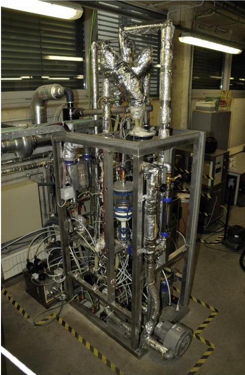
Figure 2: The TSA bench scale unit for continuous CO 2 capture from gas streams (Schöny et al., 2017)
