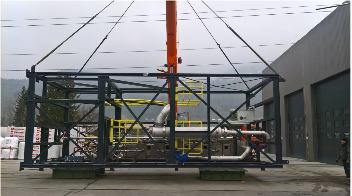
Figure 14: View of the steel structure of the TSA pilot unit container before installation of the façade (December 2017). Main pieces of equipment (adsorber and desorber column, rich and lean heat exchangers as well as flue-gas cooler and condenser) were already installed.
