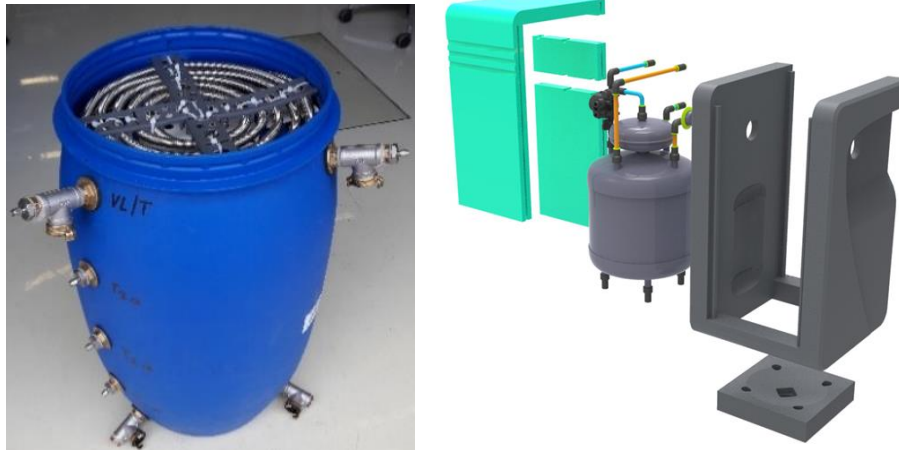
Fig. 3.11: Functional model of the heat store and concept for an all-polymeric heat store with integrated hydraulic unit and piping.
