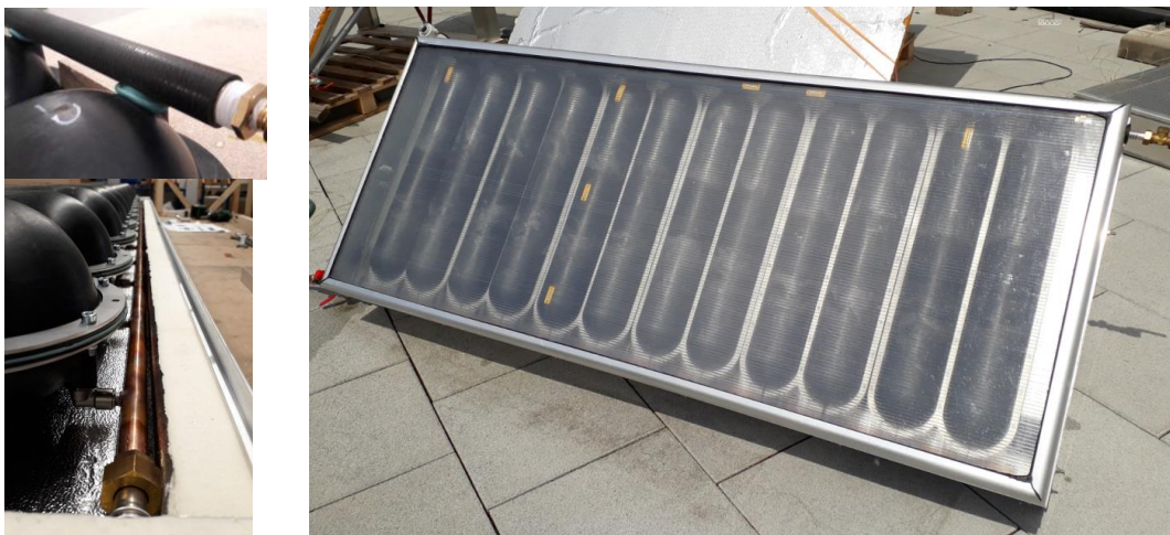
Fig. 3.12: Left: detailed construction of the single loop system. Right: Full-scale functional model out of plastic absorber-storage pipes.
