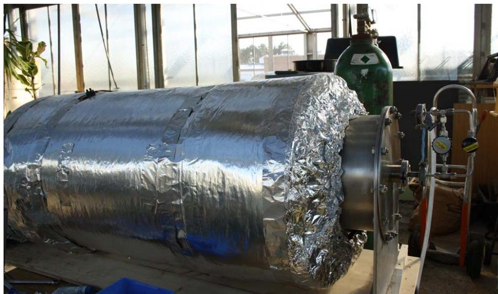
Figure 4: Pyrolysis reactor used for the biochar production of materials used later on in the microlysimeter experiment.
