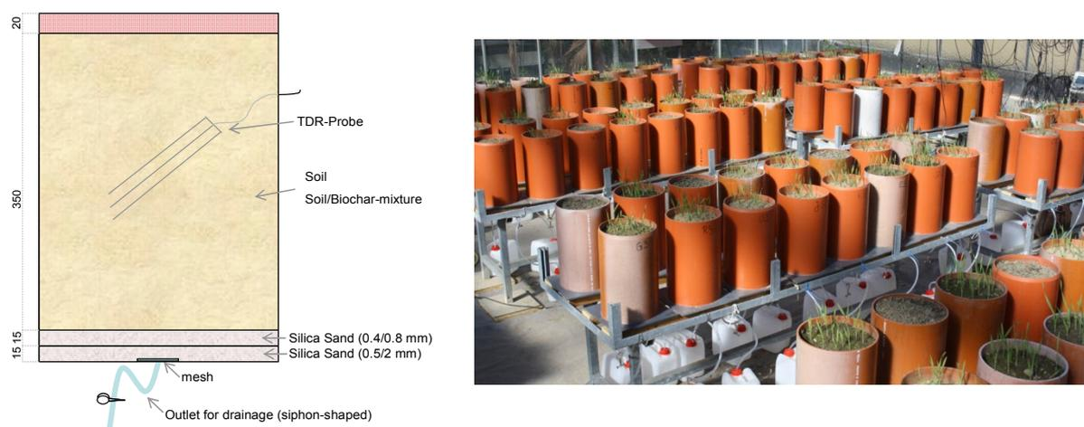
**Figure 9: Sketch of one vessel for the pot experiment; lengths in mm (left); set-up of pot experiment in the greenhouse (Photo: J. Bucker)**
