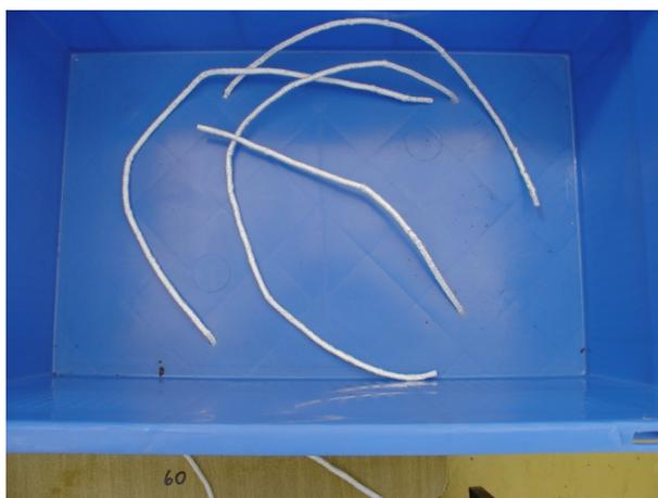
*Figure 14 Empty box and glassfiber wicks used for self irrigation of the wheat plants*
