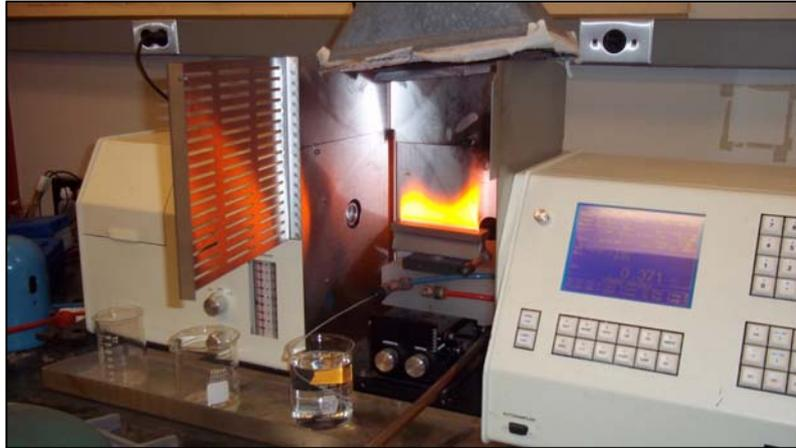
Figure 59 Atomic absorption spectrometer
