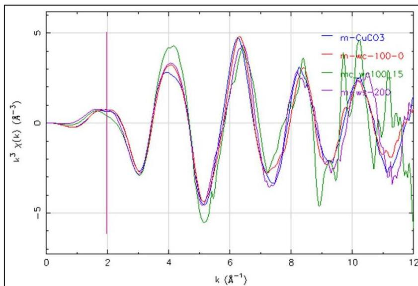
Figure 64 Derivation of EXAFS spectrum (Cu) of fresh (red line) and soil-aged (green line) woodchips-derived biochar
