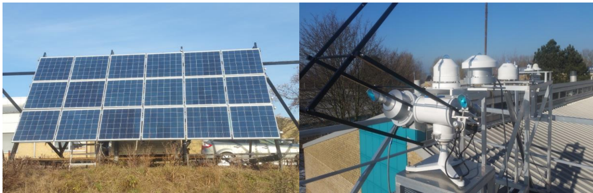
Figure 21: DTU Fotonik, Outdoor PV performance test bed (left) and weather station (right)
