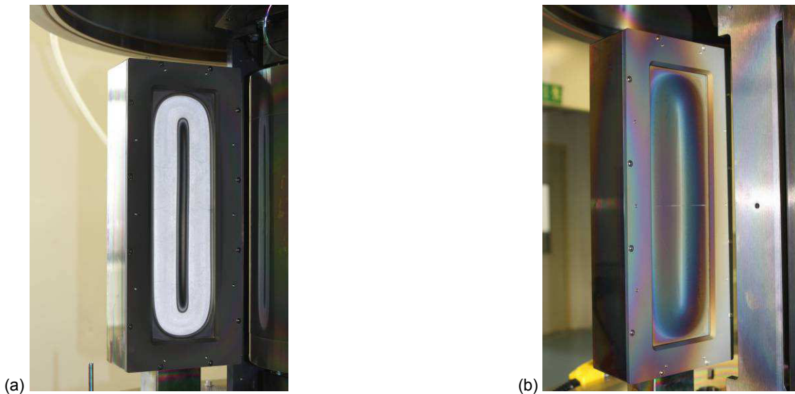
Abb. 18: Target im Roll-to-Roll-Coater: (a) ZnMg-Target (85at% Zn, 15at% Mg); (b) ITO-Target (90wt% In 2 O 3 , 10wt% SnO 2 )
