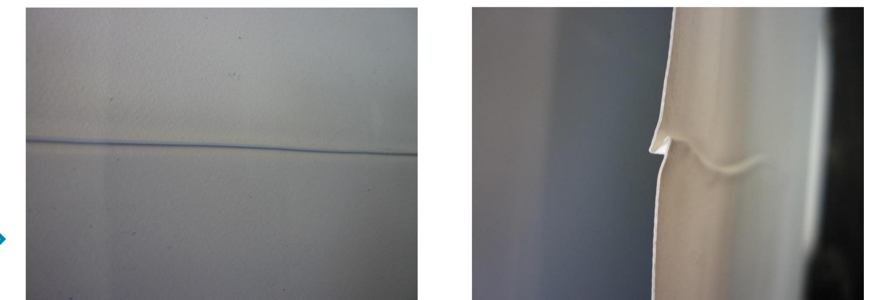
Wrinkles on PV module backsheets due to excessive anisotropic shrinkage
