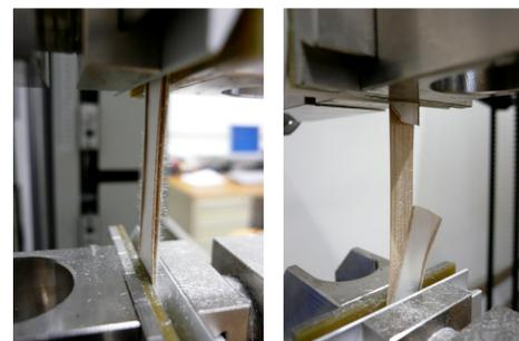
3-layer laminates with PET core layer Exposure to 85°C / 85% RH
