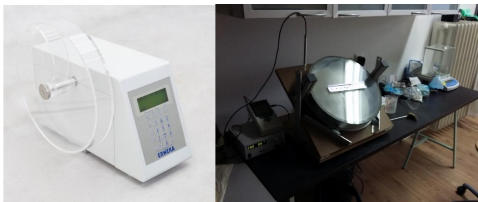
Figure 73: Friability tester used in the pharmacy (left) and experimental device (right).
