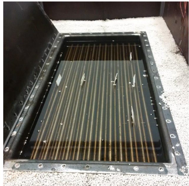
Figure 107: Left: Pure Erythritol was filled into the Kühner tube bundle storage. Right: Upon melting the material appears translucent and possesses a viscosity similar to liquid water (cf. small molecules).
