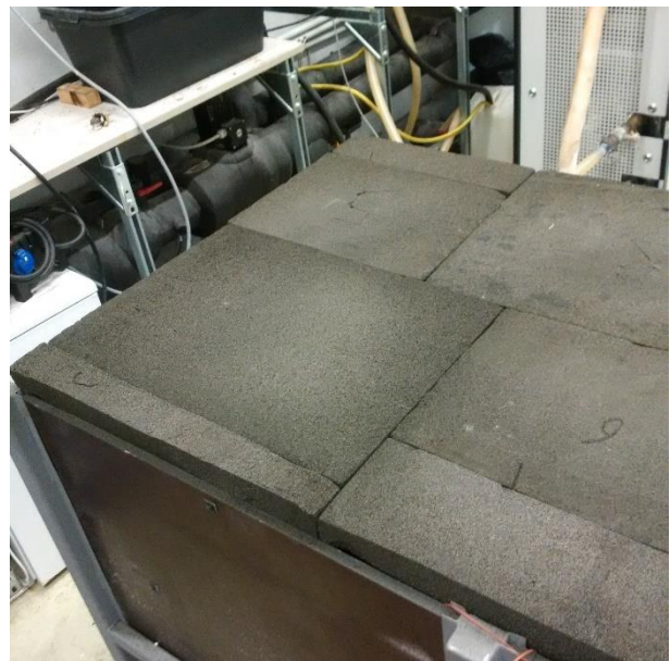
Figure 109: Left: After several filling/melting cycles the PCM compound was successfully filling the storage. The picture shows the material after re-crystallization as a black, rather solid block. Right: As top insulation we tested glass foam bricks from the company Foamglass that are thermally stable and can be easily cut to size.
