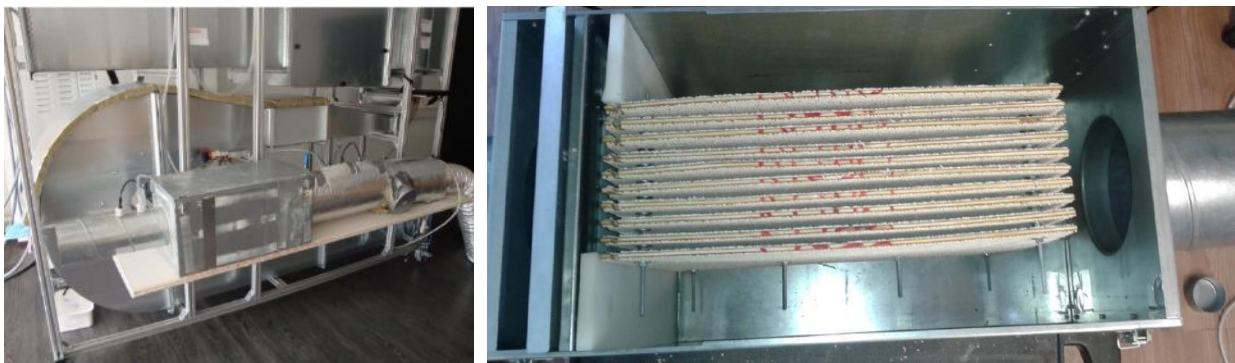
Figure 31 : ACU1 air conditioning unit to provide air at 35°C and 50%relHum (left) and specimen stacks (right).
