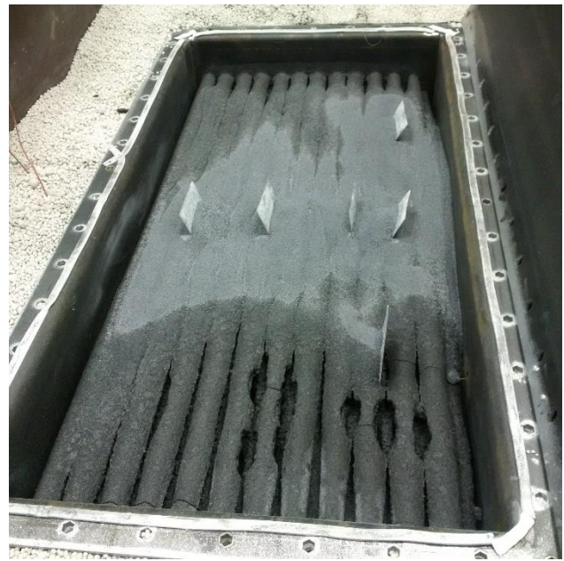
Figure 108: Left: As-delivered graphite-silica-Erythritol compound produced by Südzucker. Right: The compound was molten within the storage and possesses a very high viscosity as can be seen from the darker region where the PCM compound is already molten but still does not flow easily to the bottom of the storage. The light gray part is a PCM that is not molten yet.
