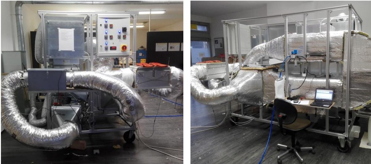
Figure 36 : Test rig extension (ACU2) for simultaneous ad- and de-sorption of the desiccant specimen
