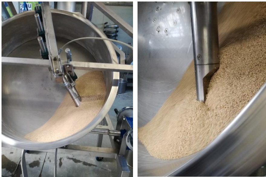
Figure 78: disc agglomeration and attrition unit with sensor (left) and detailed picture of installation in contact with the sorption material (right)
