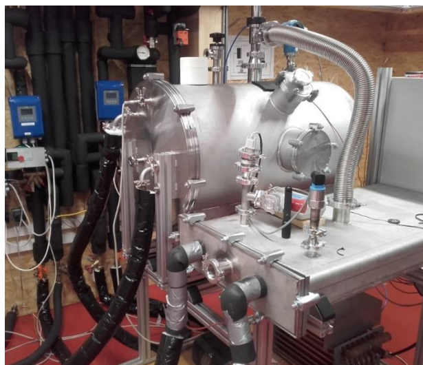
Figure 22: Test rig for the storage system including adsorber, evaporator/condenser and rectangular vessel.
