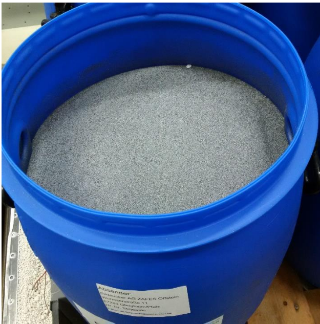
Figure 108: Left: As-delivered graphite-silica-Erythritol compound produced by Südzucker. Right: The compound was molten within the storage and possesses a very high viscosity as can be seen from the darker region where the PCM compound is already molten but still does not flow easily to the bottom of the storage. The light gray part is a PCM that is not molten yet.
