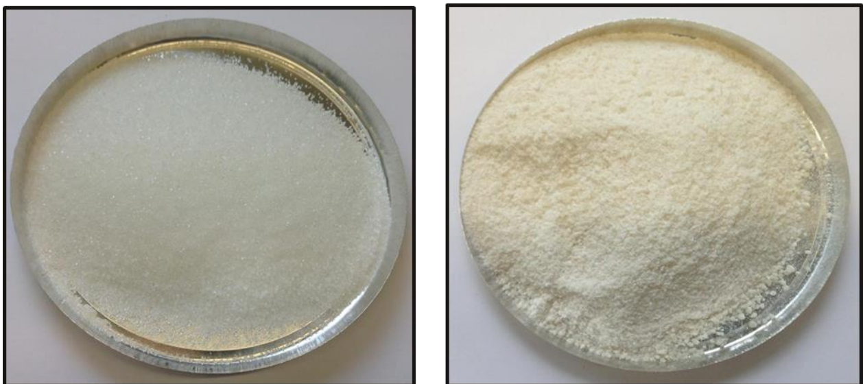
Figure 88: Erythritol sample after (left) and before (right) 100 cycles under argon atmosphere
