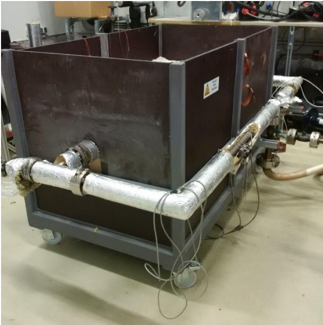
Figure 105: A special steel construction in combination with CPL boards was developed to serve as the insulation container. Foam glass aggregate from the Austrian company Geocell was used as an insulation material and was poured into the insulation containment.
