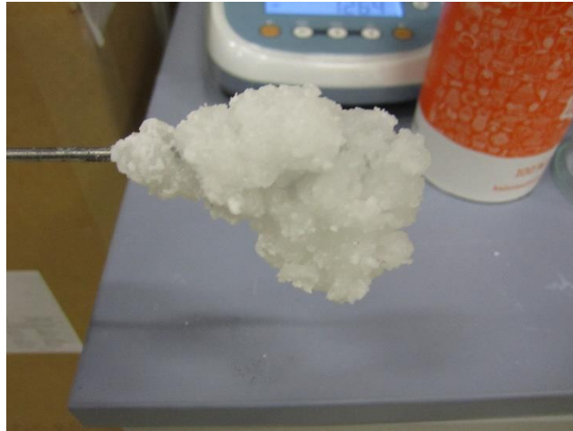
Figure 106: Fumed silica was used as a thickening additive (thixotropic agent) to prevent the de-mixing (sedimentation) of thermally conductive graphite-alditol compounds.
