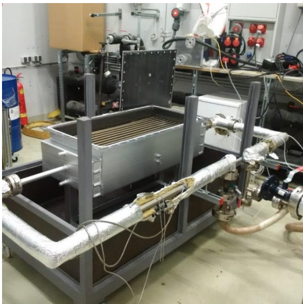
Figure 104: A dedicated test rig was designed and set up at the Thermal Storage Lab at the AIT capable of providing up to 100 kW of heating and cooling power. Various sensors were mounted around and inside the storage to characterize the PCM storages in detail.
