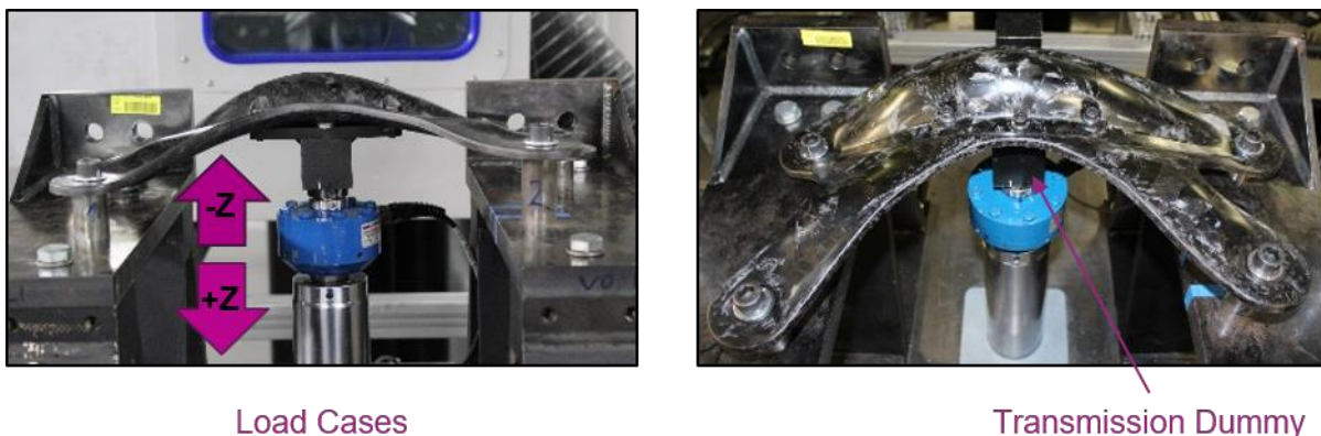
Figure 17: Component testing set-up after OEM requirements.
